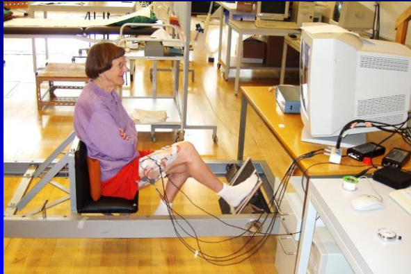
Unilateral isometric leg press test device
